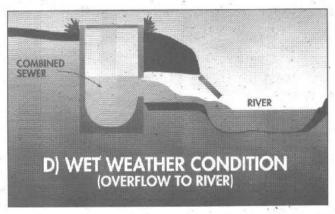
FIGURE 7: SEPARATE (A) VERSUS COMBINED (B) SEWER SYSTEM: COMBINED SEWER SYSTEMS CARRY BOTH SANITARY AND STORMWATER RUNOFF.
