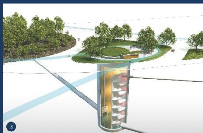
3 A Baffle Drop Structure will be used to convey flow from the existing Coxwell Sanitary Trunk Sewer into the new bypass tunnel.
